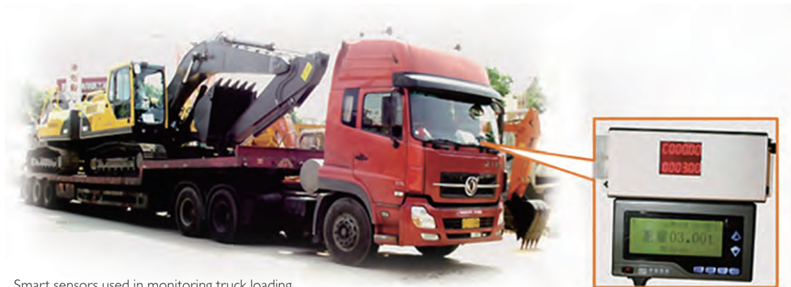
Smart sensors used in monitoring truck loading
